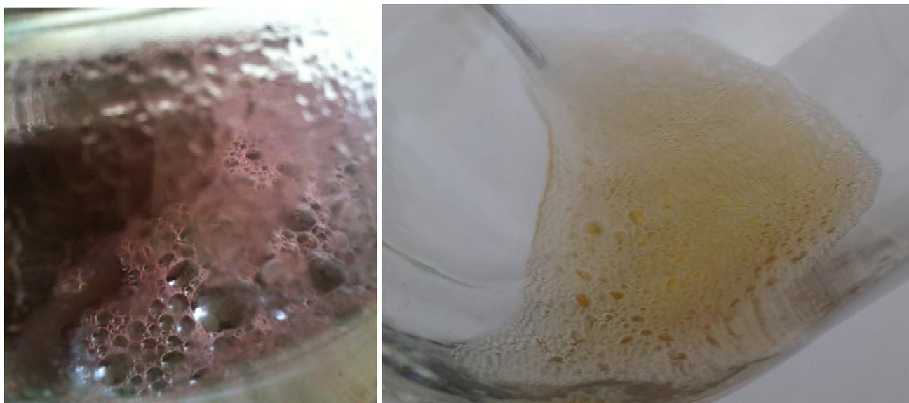
Fig. 2.50. Stable foam arising from moderate stirring of madder root powder in hot tap water (left) and from mild shaking of the same extract that had spontaneously acidified/fermented and then was acidified further by adding vinegar (right). ©AvdH
