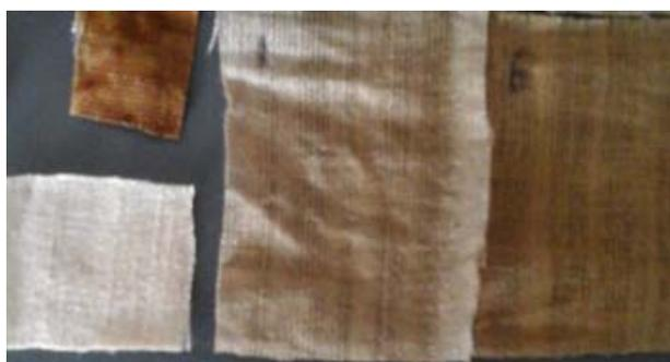
Fig. 4.33. Baking starched and not starched linen in an oven at 160 °C. Top left: starched unbleached linen, baked for 15 min, bottom left: bleached linen, baked for 15 min, centre: unbleached linen, baked for 2 hours, right: unbleached linen baked for 7 hours. ©AvdH
