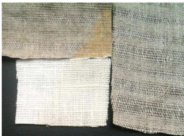
Fig. 4.32. A: Three pieces of linen scorched by simultaneously pressing the tip of a hot flatiron on them for 30 s. Top left: starched not-bleached linen, bottom left: (possibly chemically) bleached linen, right: unbleached linen. ©AvdH
