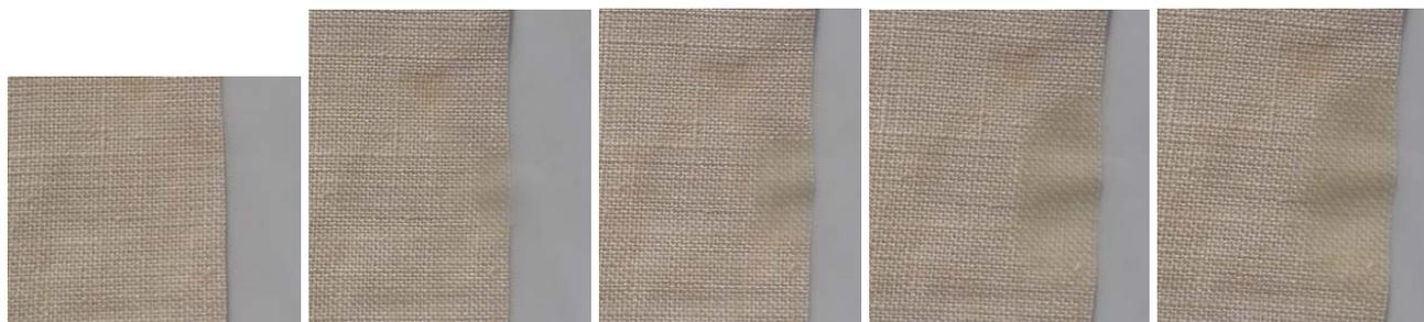
Cold water spreading in the starched-washed-and-madder-dyed linen within a minute
